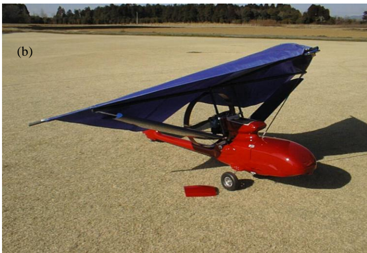
Figure 1. Three types of UAV, with wing spans of about 3 m, operated at Syowa Base (a) Operation of an engine-driven normal plane (b) Photo of a Kite plane, an engine-driven plane with a Rogallo wing (c) A gliding plane launched by a rubber balloon to 10 km in altitude.
