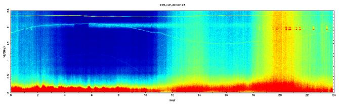
Figure 1. VLF Wide-band Spectogram obtained by the new data logger deployed in West-ongul island. This spectrum is obtained in January 23, 2013.
