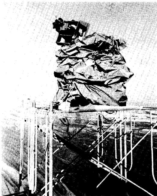
Fig. 1. Spectrometer installed on the platform above the snow surface.
