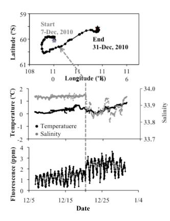
diameter) (Fig. 1). The small-scale physical disturbance of with relatively less saline surface water induced the increase of phytoplankton abundance. This suggests that the drifter developed in this study can be used for Lagrangian observations with multiple purposes, although we should pay attention to small-scale physical disturbances that affect the primary productivity.
