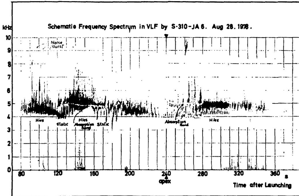
Fig. 8. The schematic frequency diagram of the VLF hiss spectra observed by S-310JA-6.
