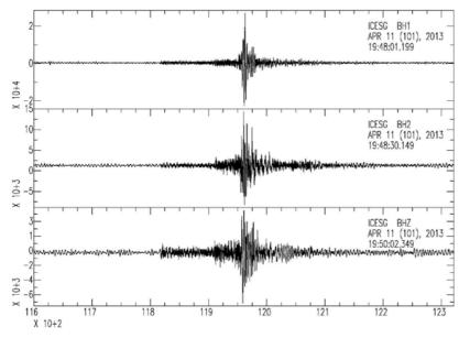
Figure 1. Three component seismograms of ICESG station for April 11, 2013 West of Greenland earthquake.
