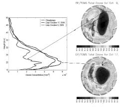
The stronger reduction of ozone column over Rio Gallegos for 2005 was produced at October 8 with total ozone column of 196 Dobson Units (DU). The lidar profile measured for this day is showed in figure above together the ozone profile measured at October 17 witch correspond to normal ozone conditions outside ozone hole (357 DU). Also in this figure the climatologic profile (black line) of SAGE II measurements is showed.
