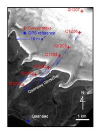
Figure 3. Locations of the survey stakes on Qaanaaq Ice Cap. Ice flow speeds are indicated by the arrows.
