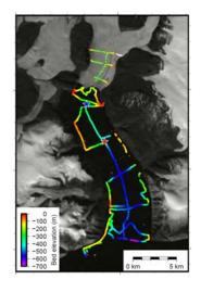
Figure 2. Glacier and ocean bed elevation measured in the field.
