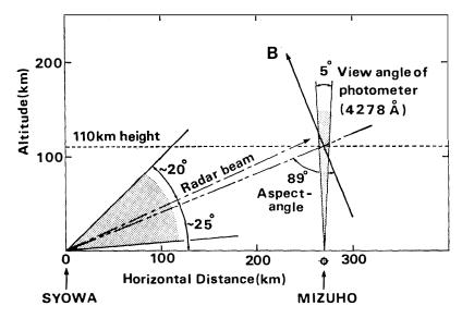
Fig. 2. Locations of the photometer and the region observed by the auroral radar. The elevation angle of the radar is  $25^{\circ}$ , the half-power beam width of the radar is about  $40^{\circ}$ , and the view angle of the photometer is  $5^{\circ}$ .
