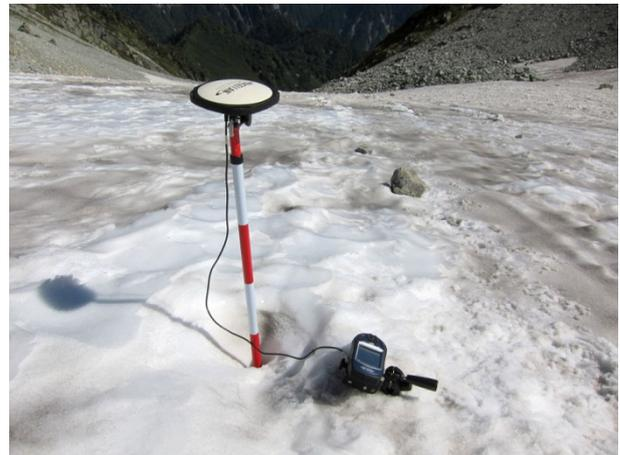
Fig.2 Stake and GPS. We installed 15 stakes on the Gozenzawa snow patch.
