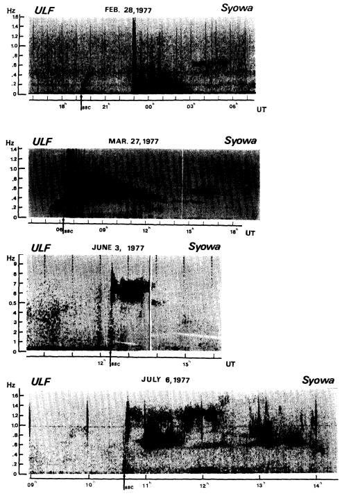
Fig. A-4. Examples of frequency-times display (f-t diagram) of ULF emissions associated with storm sudden commencements (ssz's). Onset times of ssz's are indicated by arrows in each diagram.
