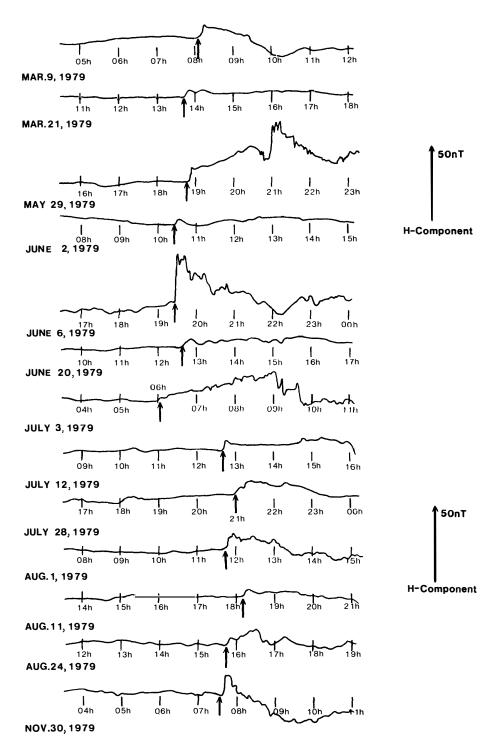
Fig. A-3. Storm sudden commencements (ssc's) records at Kakioka in 1979. Onset times of ssc's are indicated by arrows in each horizontal component trace.
