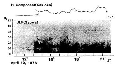
Fig. 1. Magnetic H-component variation recorded at low-latitude station, Kakioka (top) and frequency-time display (f-t diagram) of ULF emission (HM chorus) at Syowa Station (bottom).
