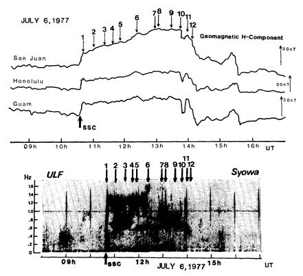
Fig. 5. Magnetic H-component variations recorded at low-latitude stations, San Juan (geomag. lat. 29.7°, long. 4.7°), Honolulu (29.6°, 328.6°) and Guam (4.2°, 214.3°) (top) and f-t diagram of ULF emissions (HM periodic emission and HM emission burst) at Syowa Station during the initial phase of a magnetic storm (bottom).
