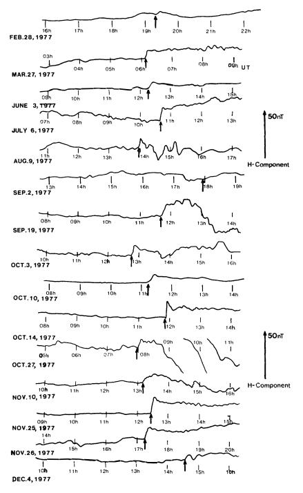
Fig. A-1. Storm sudden commencements (ssc's) records at Kakioka in 1977. Onset times of ssc's are indicated by arrows in each horizontal component trace.
