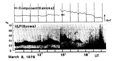
Fig. 3. Magnetic H-component variation recorded at low-latitude station, Kakioka (top) and f-t diagram of ULF emission (HM chorus) at Syowa Station (bottom).
