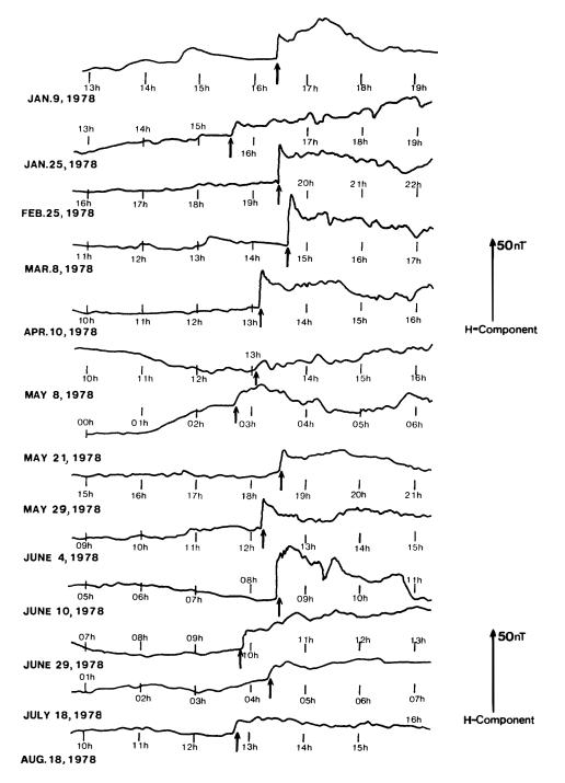
Fig. A-2. Storm sudden commencements (ssc's) records at Kakioka in 1978. Onset times of ssc's are indicated by arrows in each horizontal component trace.
