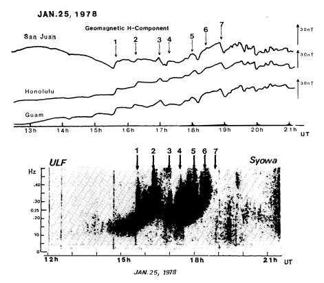
Fig. 8. Magnetic H-component variations recorded at low-latitude stations, San Juan (geomag. lat. 29.7°, long. 4.7°), Honolulu (29.6°, 328.6°) and Guam (4.2°, 214.3°) (top) and f-t diagram of ULF emissions (IPDP emission) at Syowa Station during successive si type magnetic variations.
