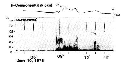
Fig. 2. Magnetic H-component variation recorded at low-latitude station, Kakioka (top) and f-t diagram of ULF emission (HM periodic emission) at Syowa Station (bottom).
