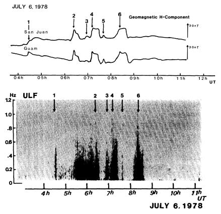
Fig. 9. Magnetic H-component variations recorded at low-latitude stations, San Juan (geomag. lat. 29.7°, long. 4.7°) and Guam (4.2°, 214.3°) (top) and f-t diagram of ULF emissions (pi-burst) at Syowa Station during successive si type magnetic variations.
