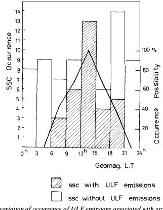
Fig. 4. Diurnal variation of occurrence of ULF emissions associated with ssc's. The unhatched histogram shows the total number of ssc's observed in the period from 1977 to 1979, while the hatched histogram shows the number of ssc's with the enhancements of ULF emissions.
