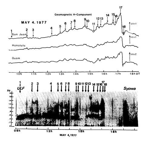
Fig. 7. Magnetic H-component variatinons recorded at low-latitude stations, San Juan (geomag. lat. 29.7°, long. 4.7°), Honolulu (29.6°, 328.6°) and Guam (4.2°, 214.3°) (top) and f-t diagram of ULF emissions (HM chorus and HM emission burst) at Syowa Station during successive si type magnetic variations.
