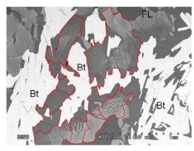
Figure 1. back scattered image of alkali feldspar partly with anti-perthitic texture and albitic plagioclase
