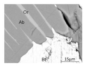
Figure 2. back scattered image of serrate projections of biotite
