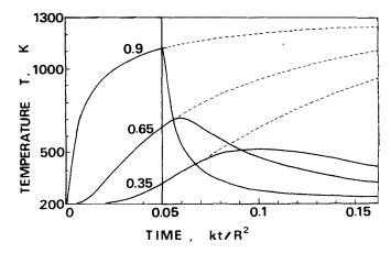
Fig. 3. Temperature variations with elapsed time  $(kt/R^2)$  for three radii (r/R) of H-chondrite parent body in the case of the Fourier number of 0.05. Numbers on curves denote r/Rand dotted lines show the temperatures for the case of infinite duration of the heat source  $(\Delta t \rightarrow \infty)$ .
