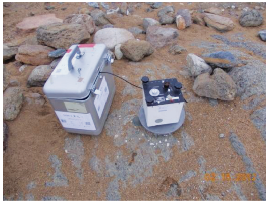
図 A-2 BM2316 点における相対重力測定 Fig. A-2. Relative gravity measurement at the BM2316 site in Syowa Station.
