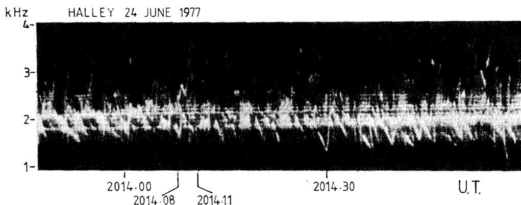
Fig. 1. The spectrogram shows a well defined array of magnetospheric lines which are gradually drifting up in frequency at  $\sim 80$  Hz/min, and lie in the frequency range 1.75–2.5 kHz. The lines trigger emission activity and show some evidence of a two hop modulation in the envelop of the wave spectrum. Local induction lines from Halley station are just visible between 1–1.5 kHz, and are regularly spaced lines of constant frequency.
