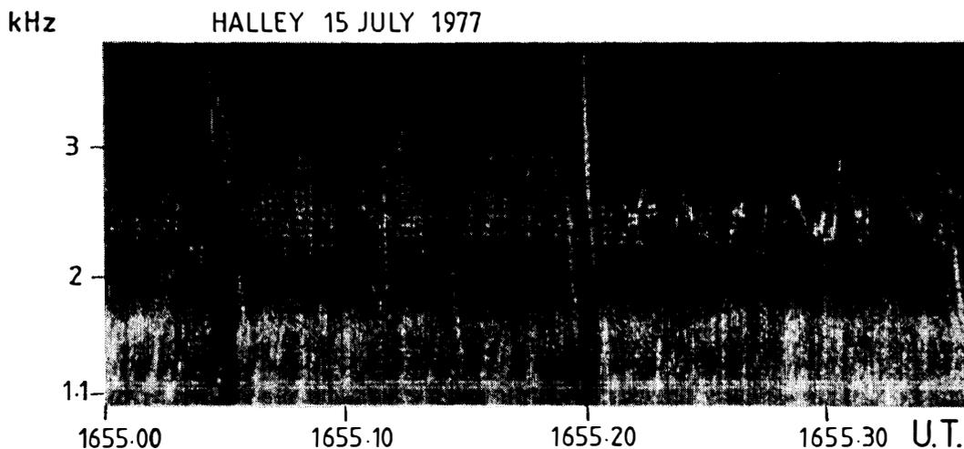
*Fig. 5. Magnetospheric line array centred on  $\sim 2.5$  kHz. Two hop amplitude modulation is visible. At 1655.05 UT and 1655.20 UT two very loud whistlers overload the receiving apparatus and cause a data drop out at lower frequencies. After 1655.22 UT the line radiation event dies out and emissions are triggered from the frequencies previously occupied by the lines.*
