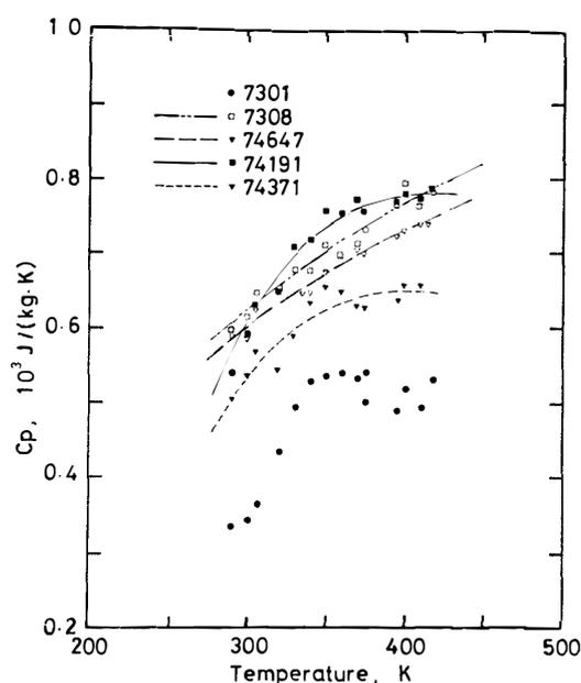
Fig. 3. Specific heat  $C_p$  versus temperature  $T$  for Yamato-7301, -7308, -74191, -74371 and -74647 in one atmosphere air.
