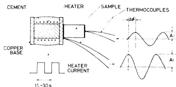
Fig. 1. Schematic diagram of the modified Angstrom method for thermal diffusivity measurement (KANAMORI *et al.*, 1968). Amplitude ratio  $A_2/A_1$  and phase shift  $\Delta\phi$  of temperatures at both ends of the sample are measured to determine diffusivity.
