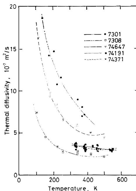
Fig. 2. Thermal diffusivity  $k$  versus temperature  $T$  for Yamato-7301, -7308, -74191, -74371 and -74647 in the vacuum condition.
