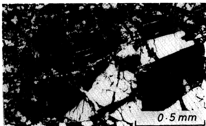
Fig. 8b. The same as Fig. 8a. Nicols crossed. The plagioclase is twinned after the pericline (75%) and albite (25%) laws.
