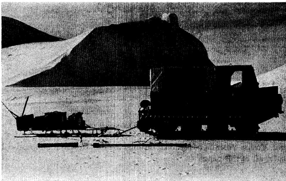
*Fig. 3. The float type snow vehicle and the light sledge using skis made by Mr. TERAJ (N.I.P.R.).
