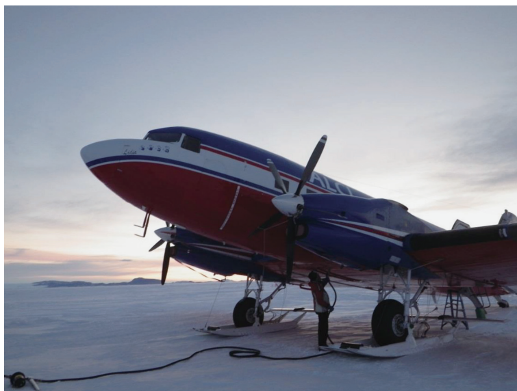
図 10 昭和基地沖海水滑走路で給油中のバスラターボ機 Fig. 10. Basler (BT-67) aircraft refueling on the sea ice runway off Syowa Station.
