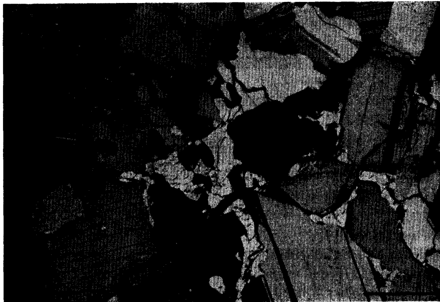
Fig. 6. Photomicrograph of the specimen 77012001. Scale bar=0.1 mm. White: scapolite, gray: plagioclase.
