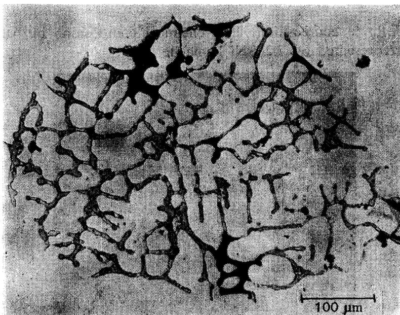
Fig. 2. Eutectic structure of schreibersite,  $(Fe, Ni)_3P$ , in Yamato-75105.
