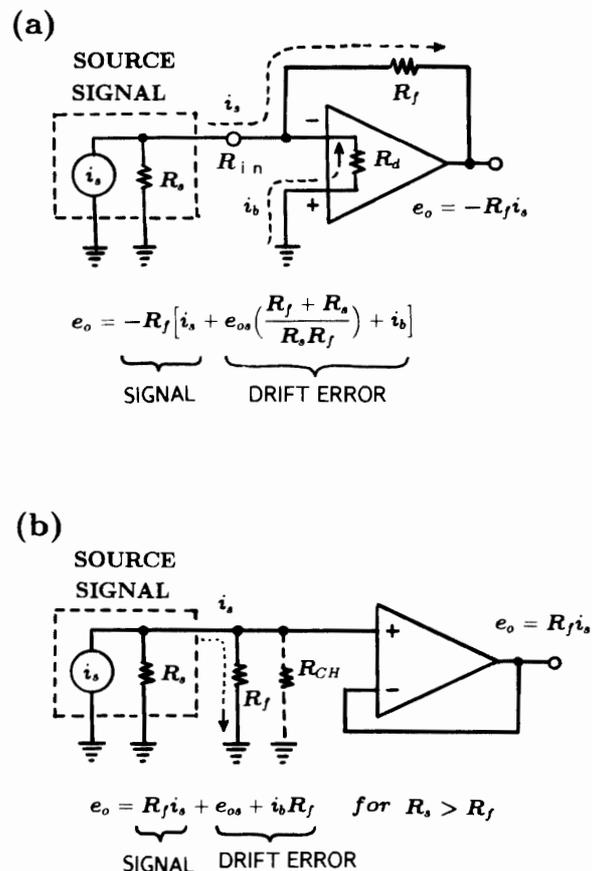
Fig. 3. Basic circuit for current meter amplifier.
