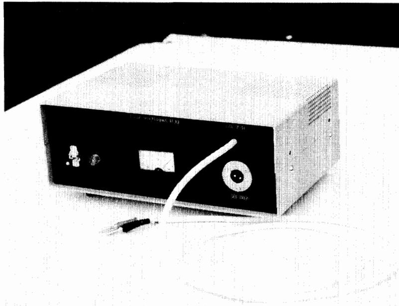
Fig. 6. An external feature of ECM amplifier.
