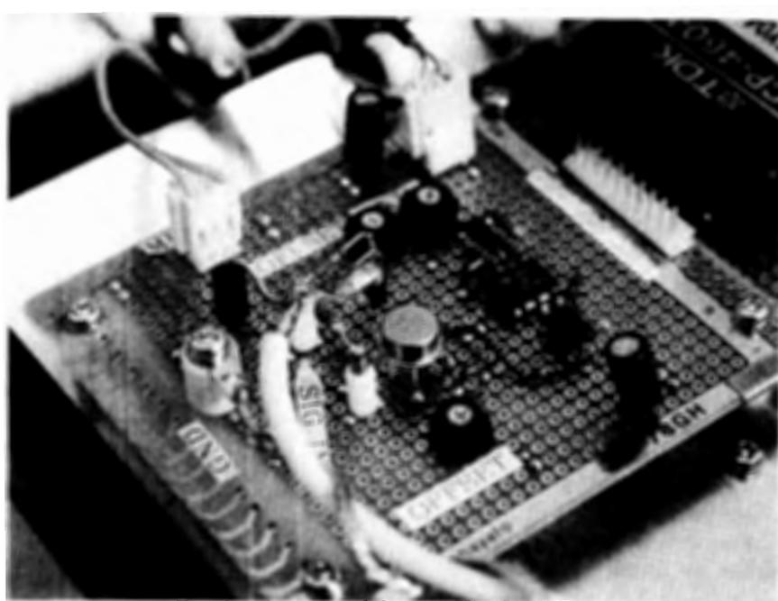
Fig. 4. An external form of HEAD-AMP.
