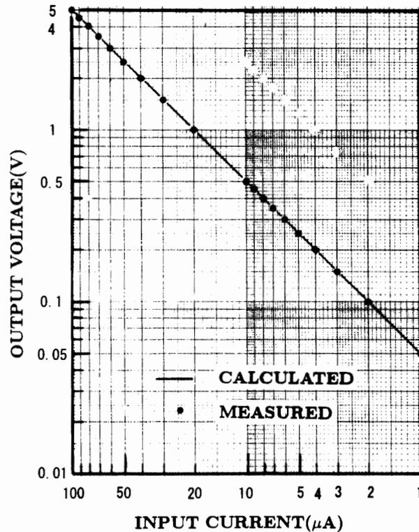
Fig. 5. Relationship between input current and output voltage.
