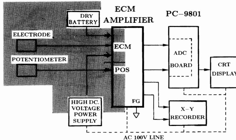
Fig. 1. Block diagram of ECM-system. The thick solid line rectangle in the center shows the ECM amplifier. In the shaded area, the circuit is "floating" when seen from the output side of the ECM amplifier.
