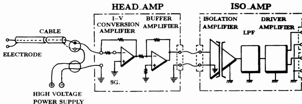
Fig. 2. Simplified diagram of ECM amplifier.
