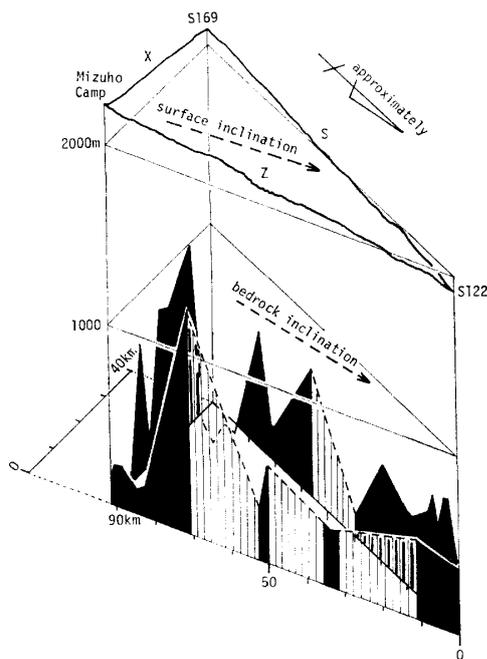
Fig. 6. Isometric drawing of the ice sheet in the region of a circuit track of Routes Z-X-S, Mizuho Plateau, in 1969-1974 (In the hatched area measurement of ice thickness is lacking. Vertical magnification to the horizontal is  $\times 45\sim 51$ , depending upon the direction).
