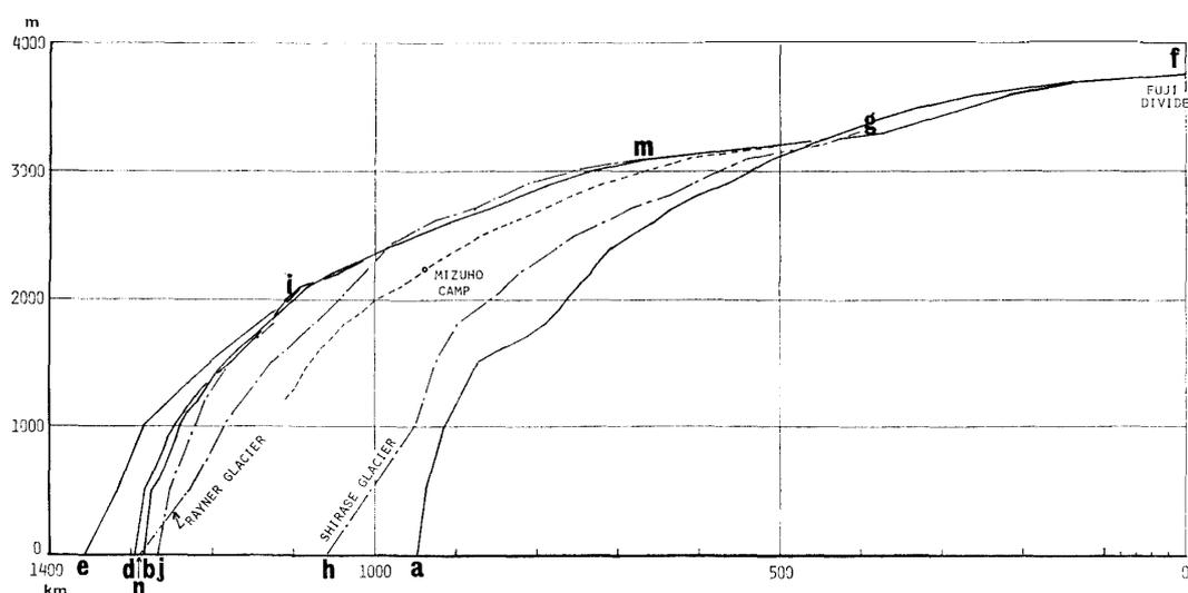
Fig. 2. Vertical profiles of the ice sheet surface along ridge and valley, in 1969-1974 (Points f, a, b, d, e, g, h, i, j, m and n correspond to those in Fig. 1).
