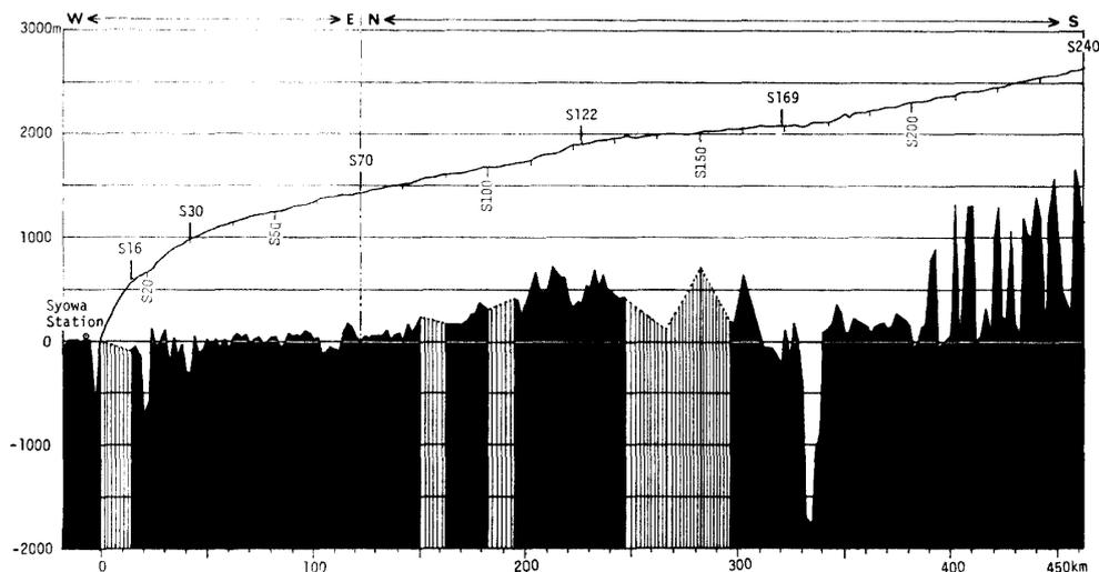
Fig. 3. Vertical cross-section of the ice sheet along Route S, from the coast to S240, Mizuho Plateau, in 1969-1974 (In the hatched area measurement of ice thickness is lacking. Vertical magnification to the horizontal is  $\times 50$ ).
