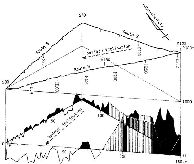
Fig. 7. Isometric drawing of the ice sheet in the region of a circuit track of Routes S-S-H, Mizuho Plateau, in 1969-1974 (In the hatched area measurement of ice thickness is lacking. Vertical magnification to the horizontal is  $\times 48\sim 51$ , depending upon the direction).
