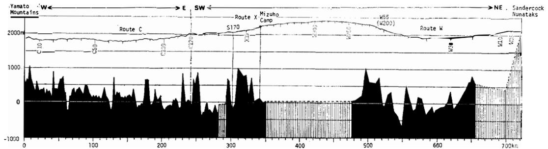
Fig. 4. Vertical cross-section of the ice sheet along Routes W, X and C, from Sandercock Nunataks to the Yamato Mountains, Mizuho Plateau, in 1969-1974 (In the hatched area measurement of ice thickness is lacking. Vertical magnification to the horizontal is  $\times 50$ ).
