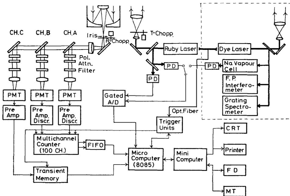
Fig. 2. Block diagram of the lidar system. The additional transmitter system based on a dye laser is indicated at the portion bounded by a broken line.
