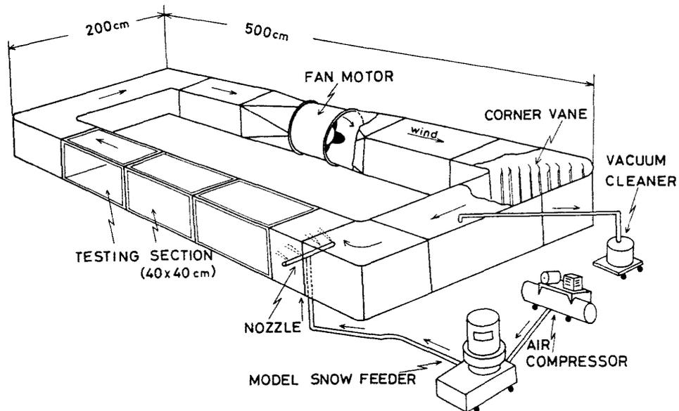
Fig. 2. Schematic view of the improved SNOWIT shown in Fig. 1.
