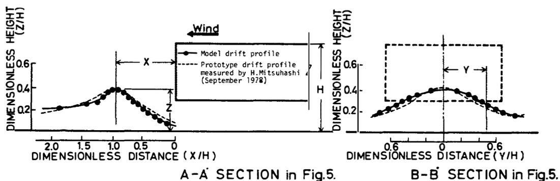
Fig. 6. A comparison of drift profiles between the model and its prototype (left: in the direction of wind; right: at right angles to it).
