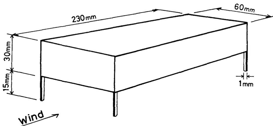
Fig. 3. Schematic view of the model building.
