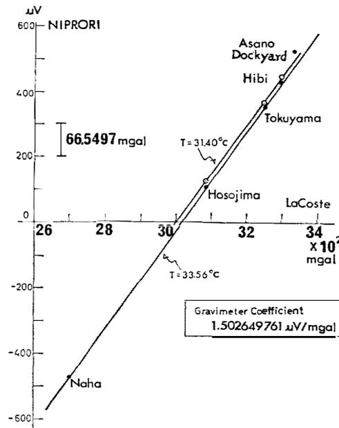
Fig. 7. Scale factor ( $\mu\text{V}/\text{mgal}$ ) of the NIPRORI gravity meter is obtained from the relationship between the output from the NIPRORI and the reading from the LaCoste & Romberg land meter. The scale factors were checked for two different temperature points  $T=31.40^\circ\text{C}$  (open circles) and  $33.56^\circ\text{C}$  (solid circles), and it was found that the ambient temperature did not affect them.
