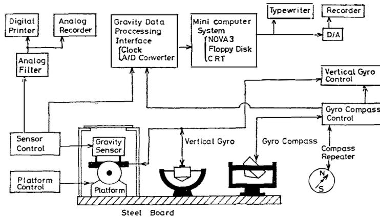
Fig. 1. Total assembly of the NIPRORI gravity meter.
