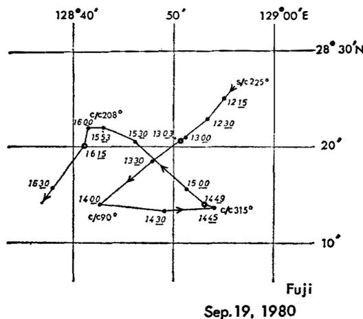
Fig. 10. Ship's track when gravity measurement was checked at the crossing of the track.
