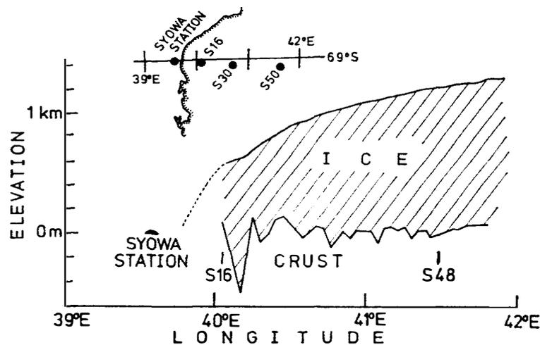
Fig. 2. Vertical sections of ice thickness along the profile.
