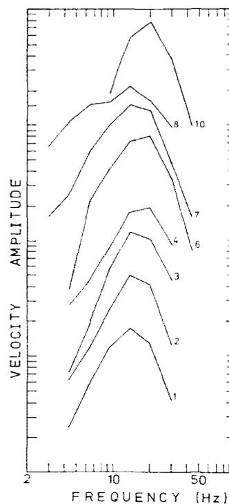
Fig. 6. Spectrum of seismogram of initial two seconds for SHOT-2.
