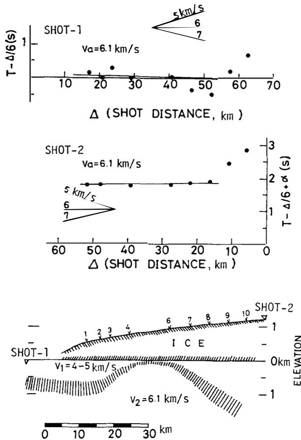
Fig. 7. Travel-time curve of SHOT-1 and SHOT-2, and vertical profile of the upper crustal structure.
