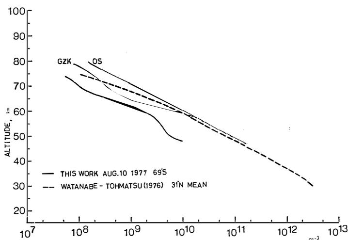
Fig. 3. Ozone concentration profile of August 10, 1977 compared with mid-latitude observed profile and theoretical profiles.
