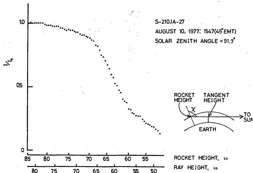
Fig. 1. Altitude profile of the relative attenuation.
