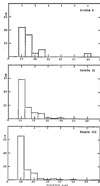
Fig. 3. Size distribution of black spherical microparticles collected from the glacier ice of the Meteorite Ice Field, Yamato Mountains.
