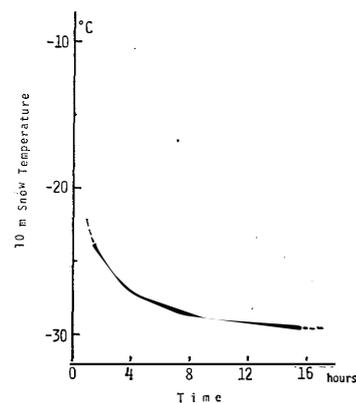
Fig. 4. The 10 m snow temperature versus the time which has elapsed after the end of drilling at Mizuho Plateau. Station, C98; Elevation, 1820 m; Date, 21–22 November 1973.
