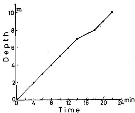
Fig. 3. Drilling rate for the firn at Mizuho Plateau. Station, H101; Elevation, 1309 m; Date, 11 November 1973; Air temperature,  $-17.5^{\circ}\text{C}$ ; Wind speed, 9 m/s; 10 m snow temperature,  $-20.1^{\circ}\text{C}$ .
