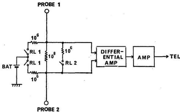
Fig. 2. Block diagram of the electric field meter.
