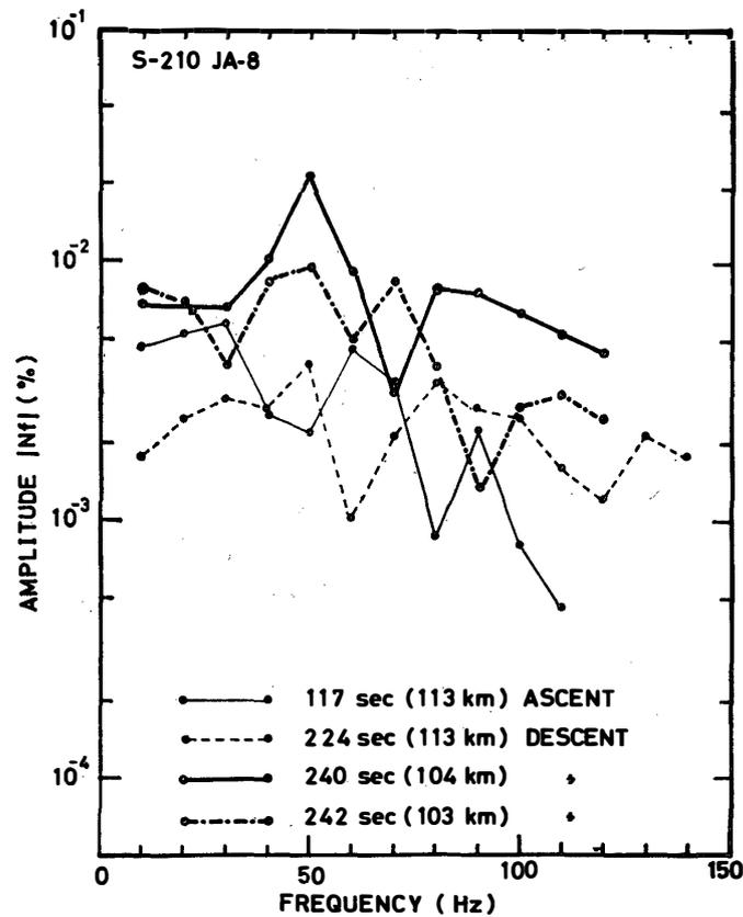
Fig. 3. Typical frequency spectrum of the irregularities detected by S-210JA-8.
