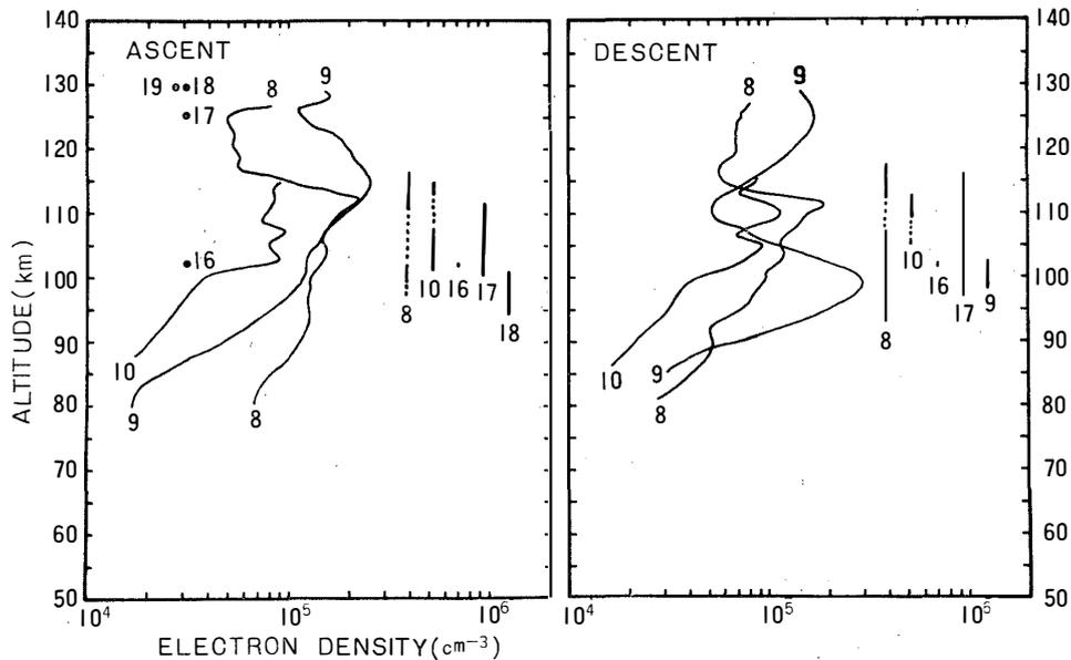
Fig. 4. Electron density profiles and altitude ranges of irregularities observed by six rockets. Number on the figure represents rocket name.
