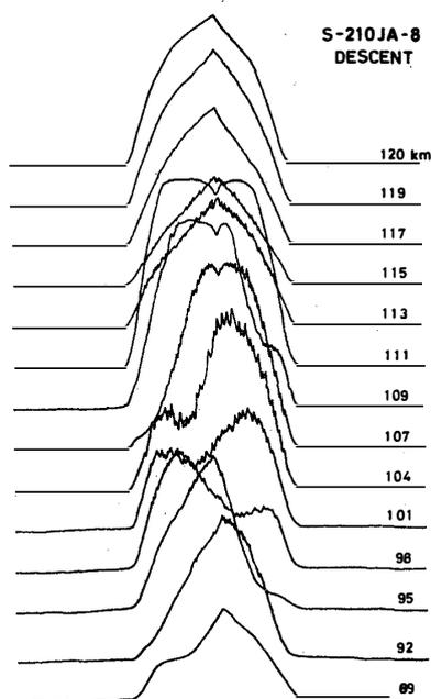
Fig. 1. Langmuir probe data at each height measured by S-210JA-8. Small irregularities exist at the saturation level of the probe current.
