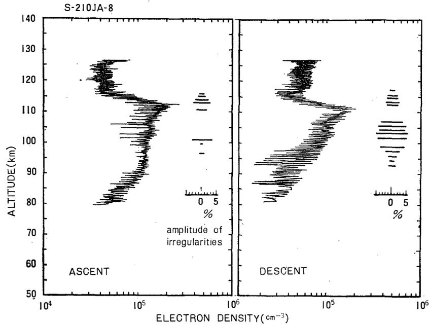
Fig. 2. Electron density profile and height variation of irregularity amplitude during the ascent and the descent of S-210JA-8.
