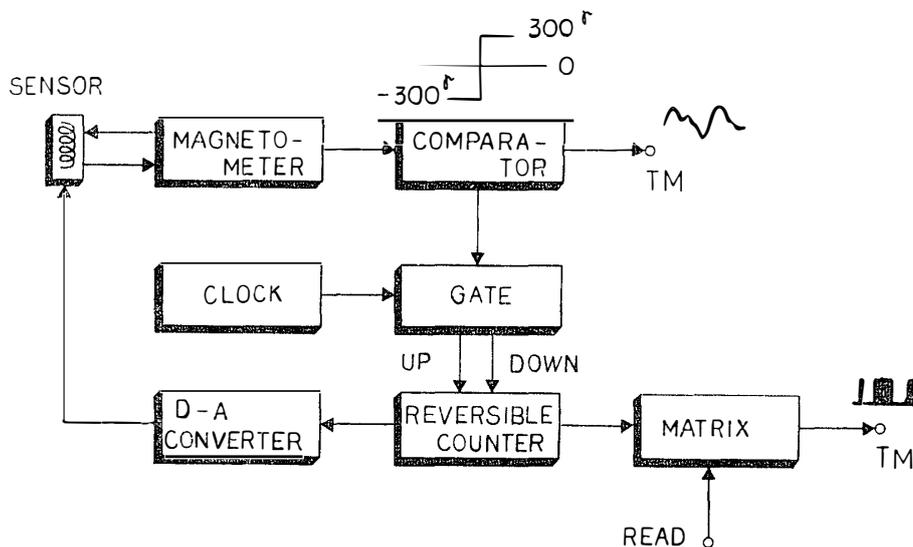
Fig. 1. Block diagram of hybrid-digital fluxgate magnetometer.
