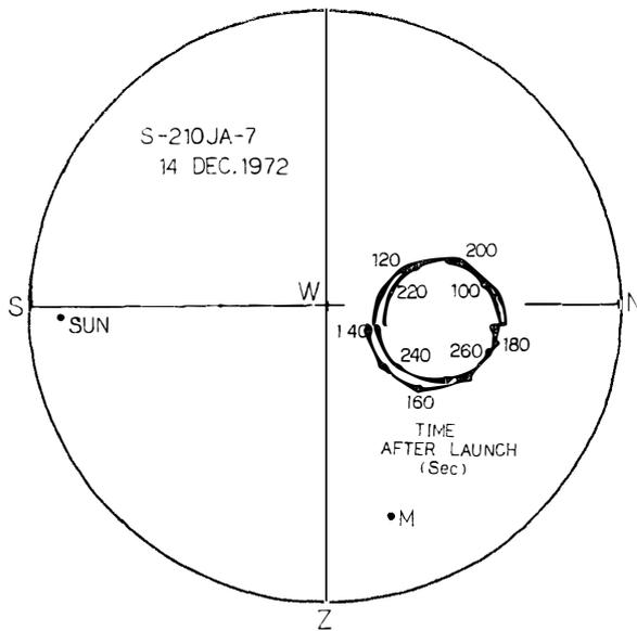
Fig. 3. Rocket axis direction on the Wuff net.
