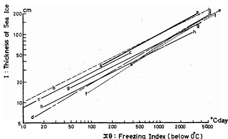
Fig. 3. Comparison of various empirical formulas relating the thickness of sea ice (cm) to the freezing index ( $^\circ\text{C}\cdot\text{day}$ ).
