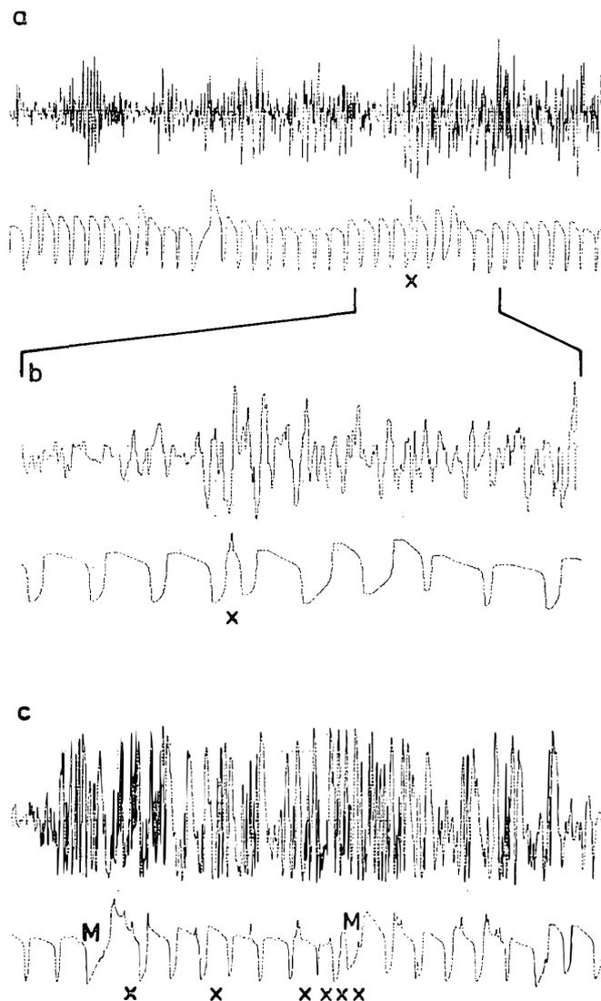
Fig. 2. Examples of deranged clock signals.  $\times$  indicates an abnormal second pulse.  $M$  indicates a minute pulse. The bottom  $c$  shows only 8-s pulses between 2-min pulses. Maximum noise-amplitudes are out of the range.
