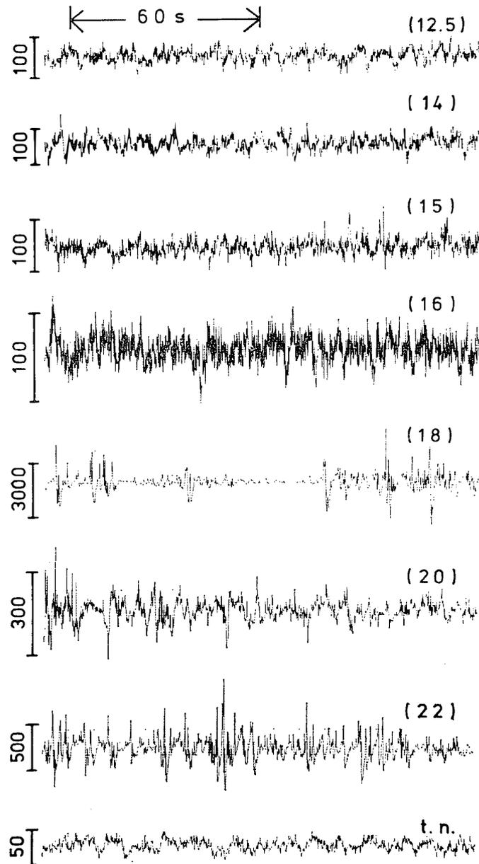
Fig. 1. Noise signals at various wind velocities. Numerals in parentheses mean the wind velocity (in m/s). The amplitude scale (in  $\mu\text{cm/s}$ ) is indicated on the left of each noise. t. n. means the tape-out noise including the electric noise generated in a data recorder and its amplitude is calculated in terms of ground velocity.
