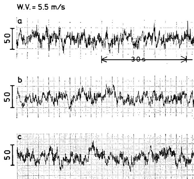
Fig. 3. Noise signals at various depths under a wind velocity of 5.5 m/s. a, b and c are recorded at depths of 0, 3 and 5 m, respectively. On the left side of each signal, amplitude scales (in mV) are indicated, which are measured on reproduced signals.
