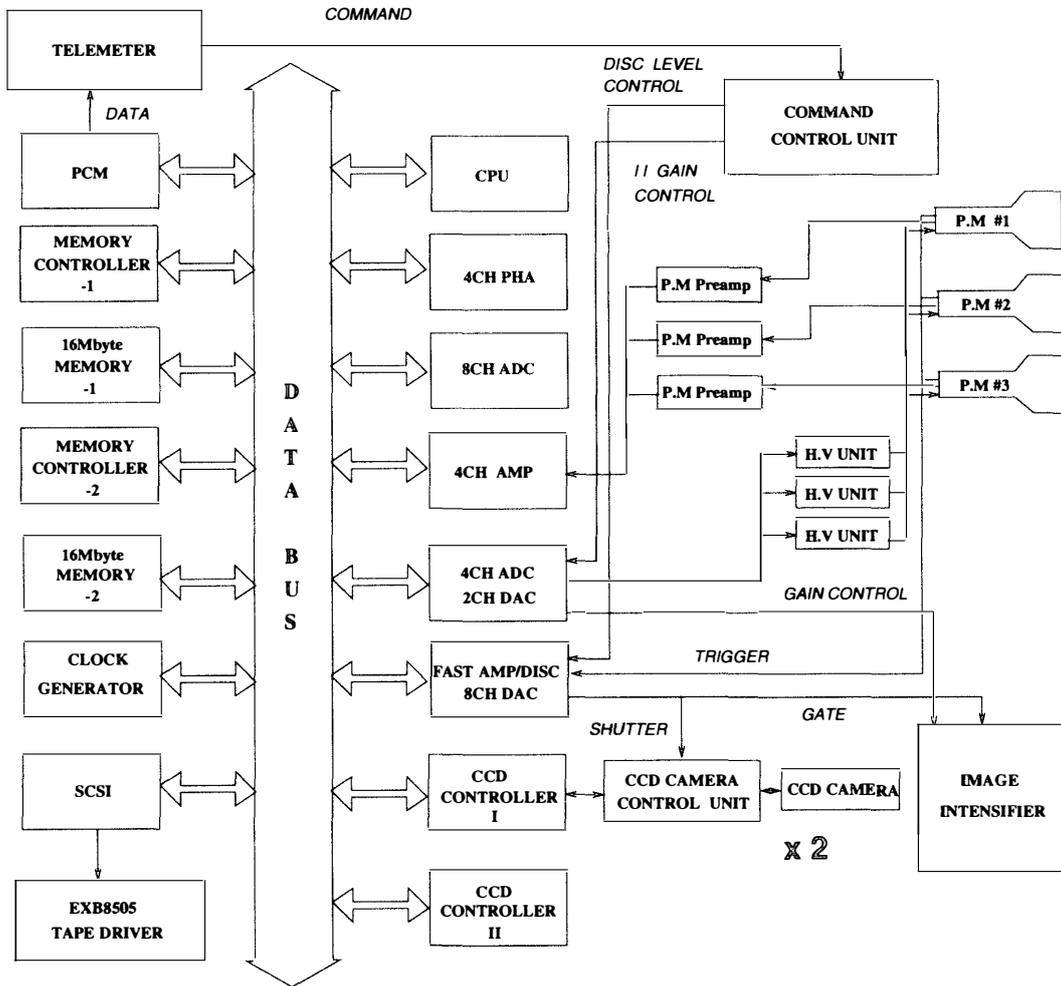
Fig. 3. Block diagram of the electronics system of the BETS detector. Similar system will be used in the instrument for PPB.
