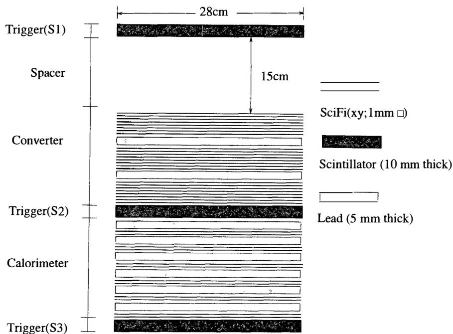
Fig. 2. Schematic side-view of the detector.
