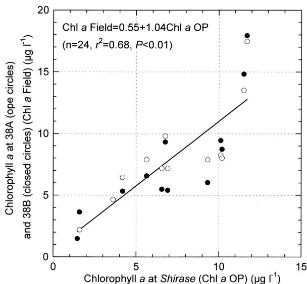
Fig. 4. Relationships between chlorophyll *a* concentrations observed aboard the *Shirase* using the surface seawater monitoring system (Chl *a* OP) against field observations (Chl *a* Field) at Sites 38A (open circles) and 38B (closed circles) (Odate, unpublished data).
