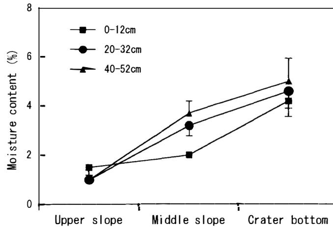
Fig. 2. Depth profile of soil moisture content on the upper slope, middle slope and crater bottom at the Hiei second crater. The soil moisture was measured by using a handy TDR with 12 cm long sensor after 7 successive rainless days.
