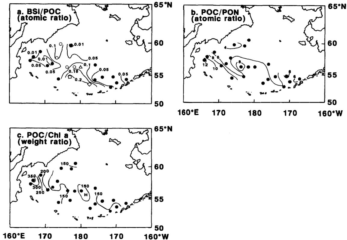
Fig. 5. Regional variations of BSi/POC (a), POC/PON (b) and POC/Chl *a* (c) at the surface. In Fig. 5a, open symbols indicate stations with values exceeding the averages.  $\triangle$ : BSi/POC=0.14;  $\diamond$ : BSi/POC=0.20;  $\square$ : BSi/POC=0.21. Ranges and averages are shown in Table 1.
