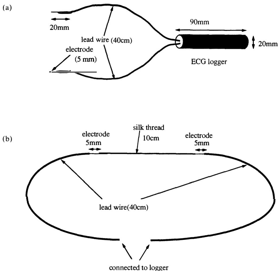
Fig. 1. The ECG logger and the electrodes used for Adélie penguins (a) and hens (b).
