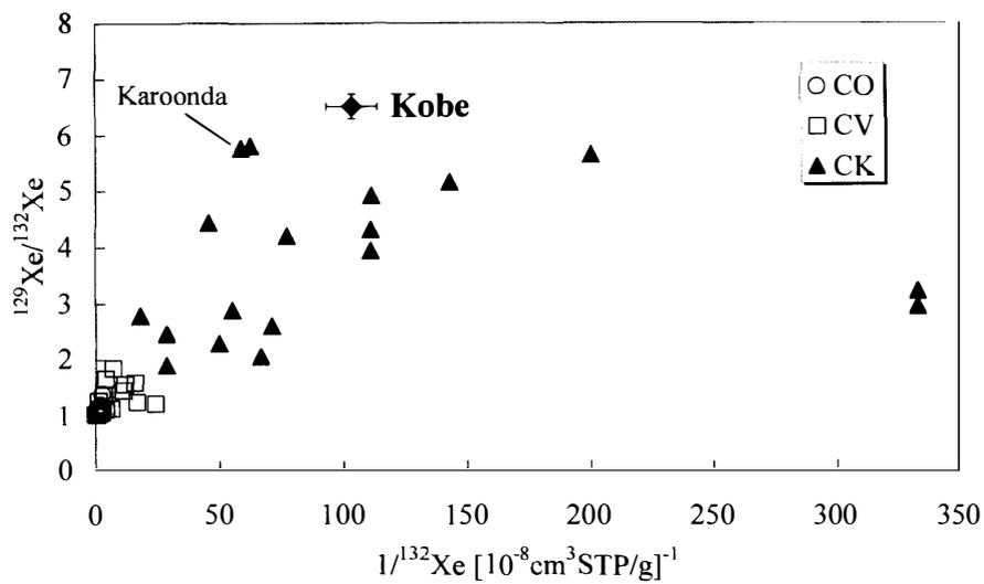
Fig. 2. A  $^{129}\text{Xe}/^{132}\text{Xe}$  vs.  $1/^{132}\text{Xe}$  plot. CK chondrites have low  $^{132}\text{Xe}$  concentrations and pronounced excesses of  $^{129}\text{Xe}$  compared with CO and CV chondrites. Kobe has the highest  $^{129}\text{Xe}/^{132}\text{Xe}$  ratio in this diagram. The data of this diagram, aside from the data for Kobe, are derived from Scherer and Schultz (2000).
