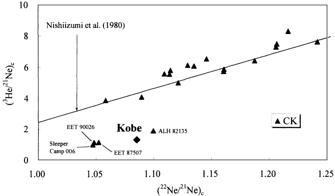
Fig. 3. A  $(^3\text{He}/^{21}\text{Ne})_c$  vs.  $(^{22}\text{Ne}/^{21}\text{Ne})_c$  plot (so-called Bern Plot) for CK chondrites. The solid line is a best fit for ordinary chondrite data (Nishiizumi et al., 1980). Kobe and some CK chondrites plot considerably below this line, which indicates  $^3\text{He}$  loss. Noble gas data in this diagram, aside from Kobe data, are derived from Shima et al. (1973), Wieler et al. (1985), and Scherer and Schultz (2000).
