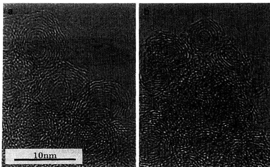
Fig. 3. HREM images of (a) the granular-QCC and (b) the dark-QCC. The materials are an aggregate of onion-like particles. EM images are shown on the same scale.
