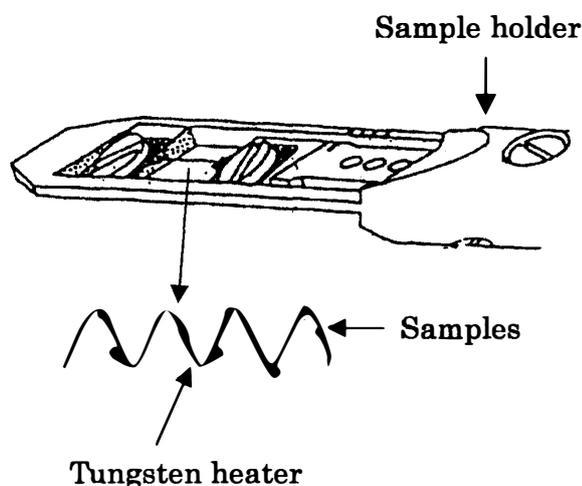
Fig. 2. Schematic representation of the sample holder used in the *in-situ* observation. QCC samples were directly mounted on the conical tungsten heater. Samples are shown by filled circles.
