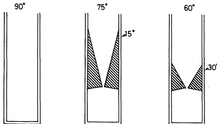
Fig. 1. Vertical section of settling tubes with and without cone. The values above each tube indicate the angle of cone-wall from the vertical wall. Bottom diameter of cone is 3 mm.
