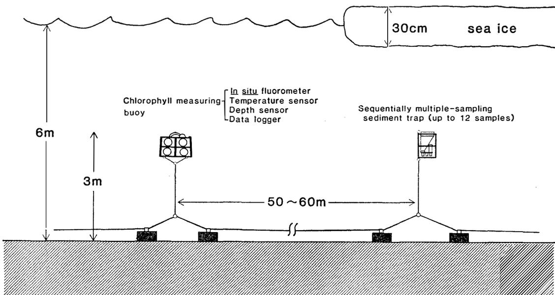
Fig. 1. Mooring array of the chlorophyll-measuring buoy and the sediment trap in a lagoon, Saroma Ko, Hokkaido, Japan.
