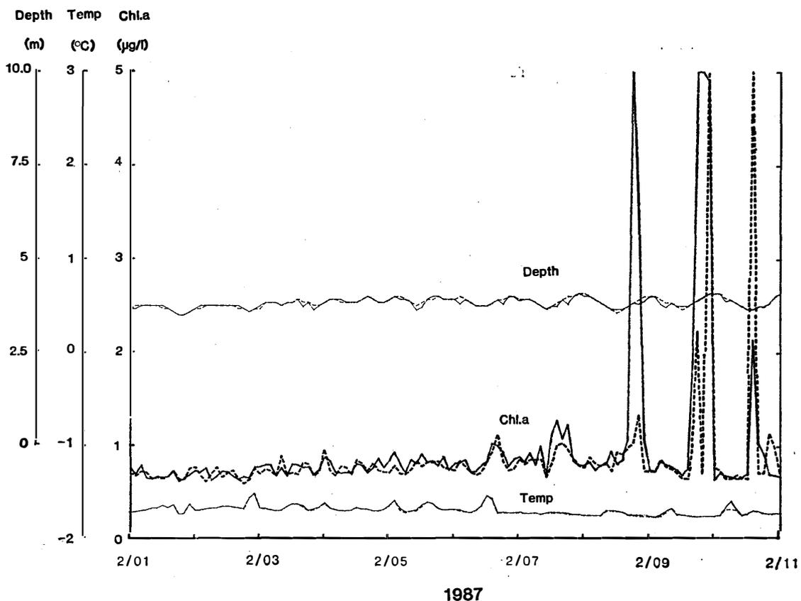
Fig. 3. Time series data over 10 days on depth, temperature and chlorophyll *a* between 1 and 10 February 1987 in lagoon Saroma Ko, Hokkaido, Japan. Data obtained before, and after, washing the window of fluorometer are shown by solid, and dashed lines, respectively.
