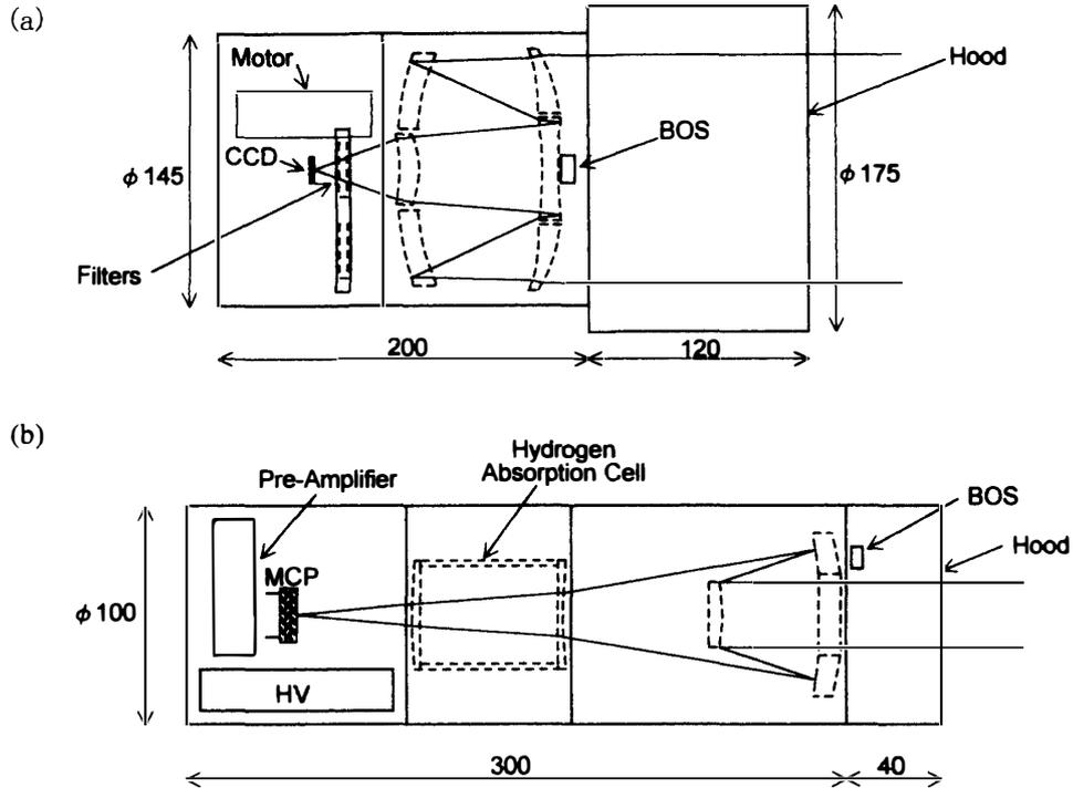
Fig. 1. Schematic drawings of (a) UPI-TVIS and (b) UPI-TUV. Scales are in mm.
