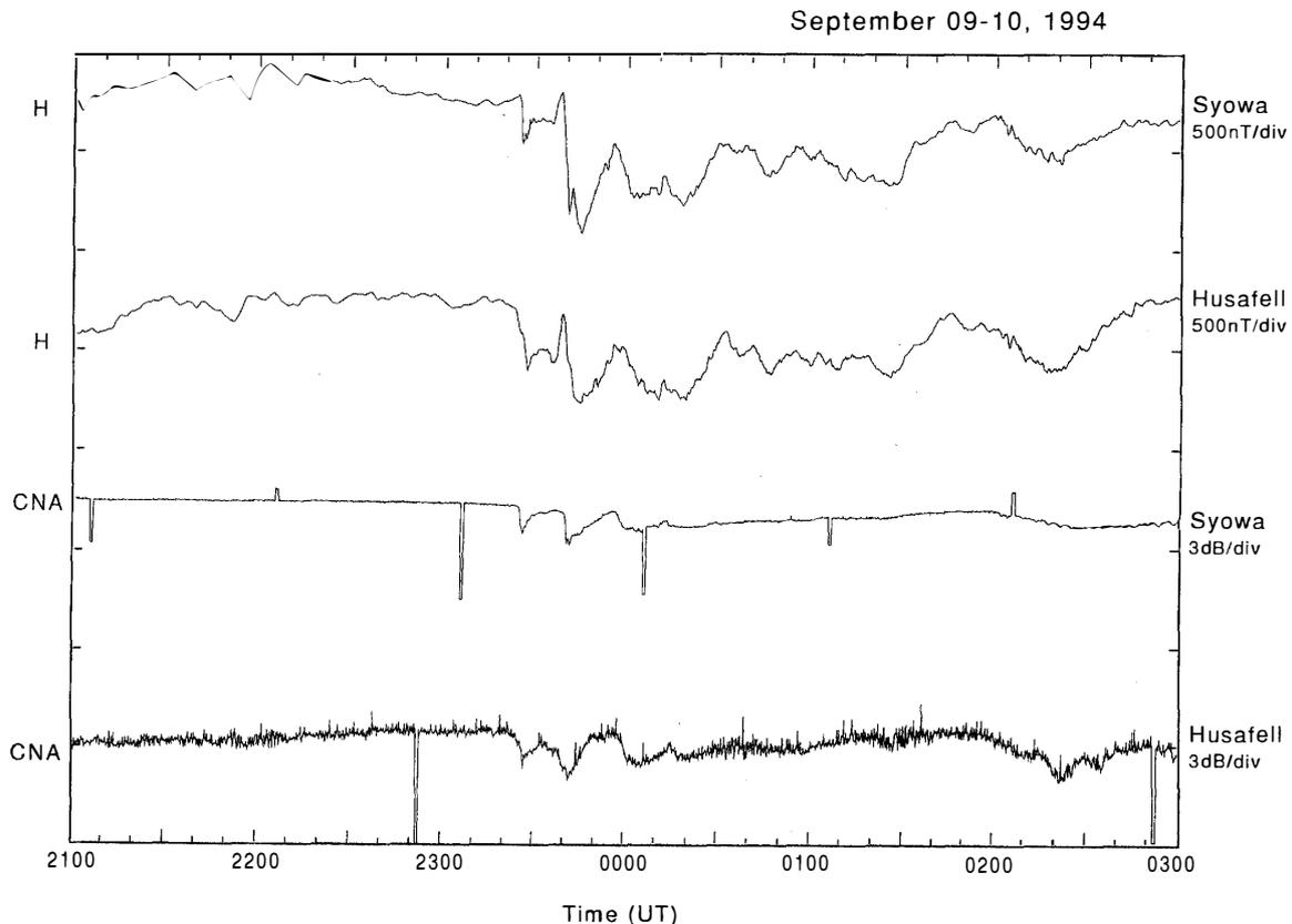
Fig. 1. The  $H$  component of magnetic variations and the CNA (Cosmic Noise Absorption) observed simultaneously at Syowa Station in Antarctica and Husafell in Iceland. We are interested in here particularly in the time interval of 0013–0021 UT.
