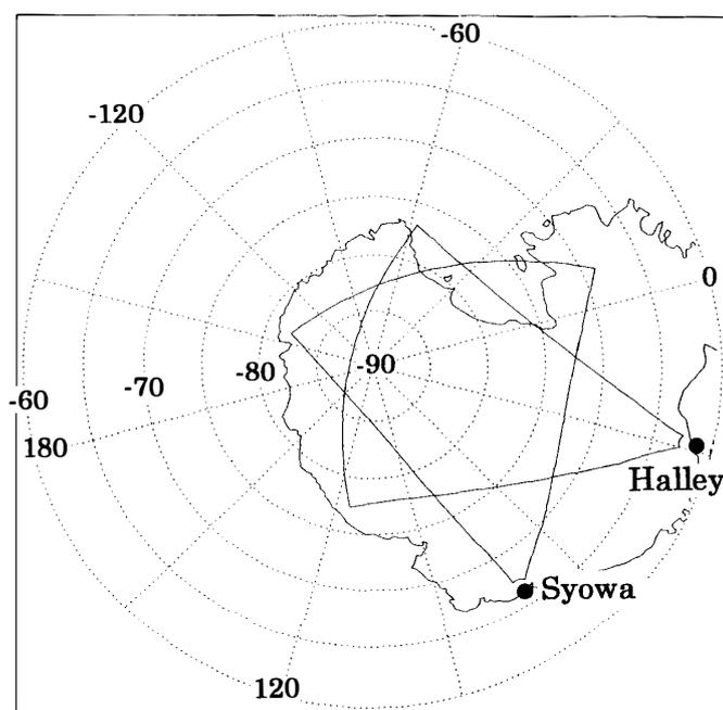
Fig. 1. Fields of view (FOV) of Syowa Station and Halley HF radars in magnetic coordinates. Each FOV is covered with sixteen beams.
