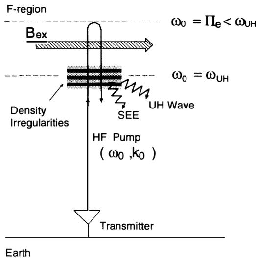
Fig. 1. Schematic of the typical ionospheric heating situation.
