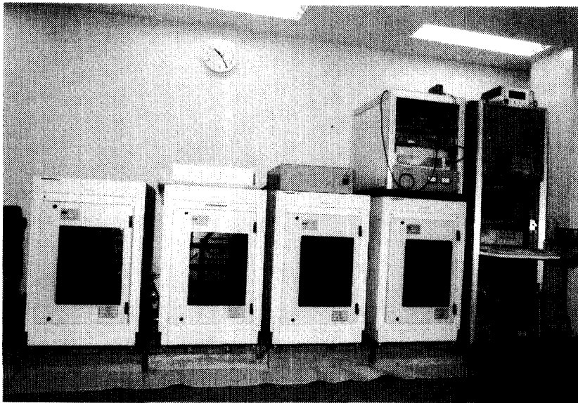
Fig. 3. Scanning-beam VHF auroral radar system showing four power amplifiers, a receiver and a signal processing PC.
