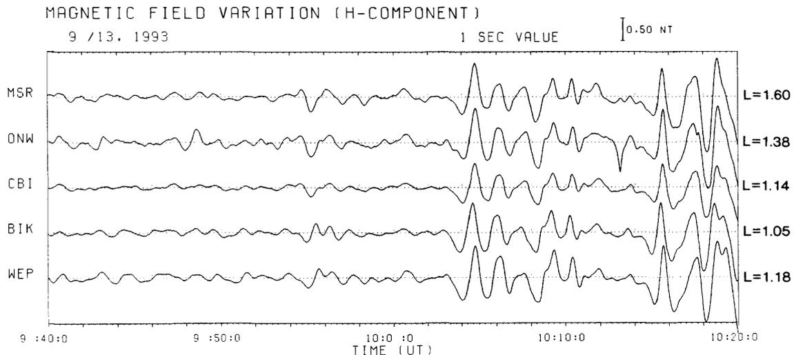
Fig. 3. Pulsations in the  $H$  component magnetic field observed at low-latitude stations for 0940 UT–1020 UT on September 13, 1993. These stations are the same as those shown in Fig. 2 except for BSV which is omitted due to a high noise level. The peak period of the band pass filter used in this plot is 80 s, while the gain of the filter becomes 0.5 at the periods of both 40 and 160 s.
